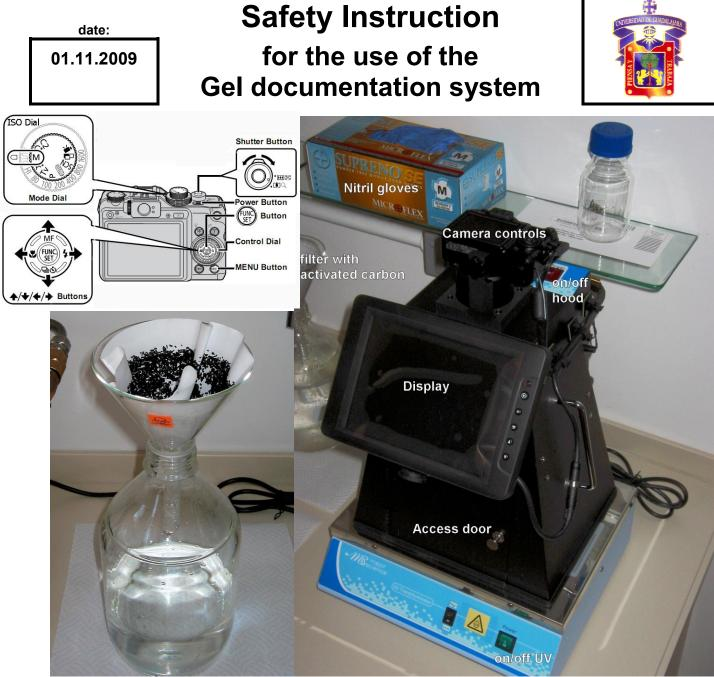
Camera has Tele-converter (2.2x) and band-pass filter for EtBr attached Band-pass filter let pass only orange light, emitted from EtBr when excited For non-UV gel documentation, this filter has to be removed and use epi-white light source
